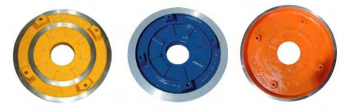
Frame plate liner insert is also one of wet parts of slurry pumps, someone also call it as slurry pump back liner based on it position in slurry pump. It forms a pump chamber with throat bush and volute liner where the slurry would flow through them.
