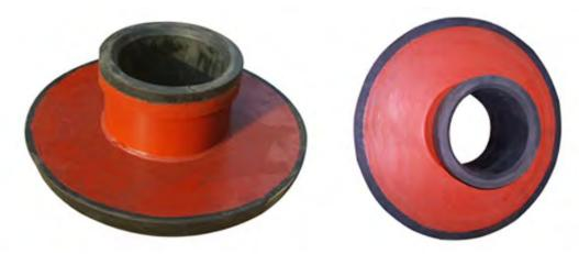
Rubber slurry pump throat bush is used to deal with the corrosive slurry with blunt particles. They are made of natural rubber, synthetic rubber, EPDM Rubber, Nitrile Rubber, Fluoroelastomer or any other as you required.
